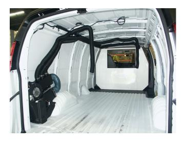
Route HVAC 2 1/2" blower hoses to the approximate locations with tape along ceiling where they will be installed into the ceiling insert after Kwik-Kit insert is installed. Mount hoses with wire ties at wall and ceiling corners only. Leave enough slack to reach hoses for permanent mounting.
